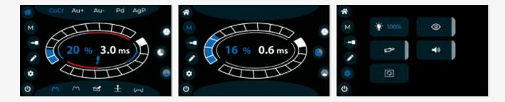
Optimised settings menu with practical additional functions such as the enhanced micro mode, the retention welding mode, or the fixation welding function.
